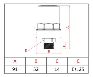
The WHS hammer arrestor can be described as cylinder divided in two chambers, separated by a disk, each kept fully sealed by an O-ring. As well as exploiting the compressibility of air, the "closed" chamber is equipped with a spring, which absorbs and evens out the sudden increase in pressure that occurs in the "open" chamber (the one connected to the system) during water hammer propagation.
