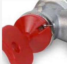
2. Set the R73PY010 key on the bonnet stem, fitting it in the only position allowed (letter "N" visible from the slot of R73PY010 key and facing the reference "A" on the valve body). Turn the bonnet stem using the key R73PY010 until the desired presetting number number appears from the slot of the key.
