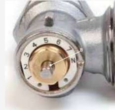
3. Remove the wrench R73PY010, the stem "B" will be on the desired pre-setting position, marked by the number on the valve ring. Adjustment positions 0,5 (single notch) - 1 - 2 - 3 - 4 - 5 - 6 - 7 - N (N = fully open).
