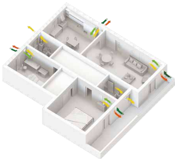
ALTERNATED SIMPLE-FLOW SYSTEM WITH STATIC HEAT RECOVERY.
