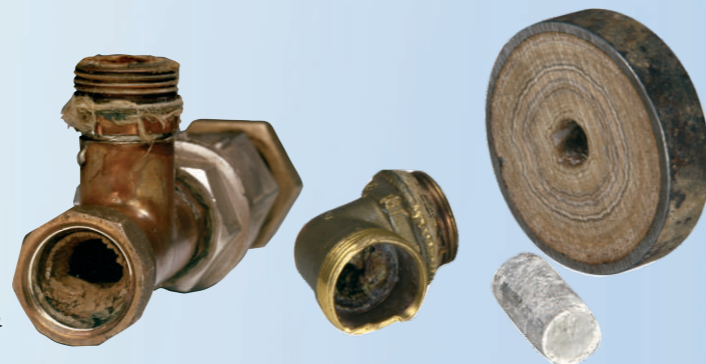
Examples of pipes and fittings exposed for a long time to limy water.
